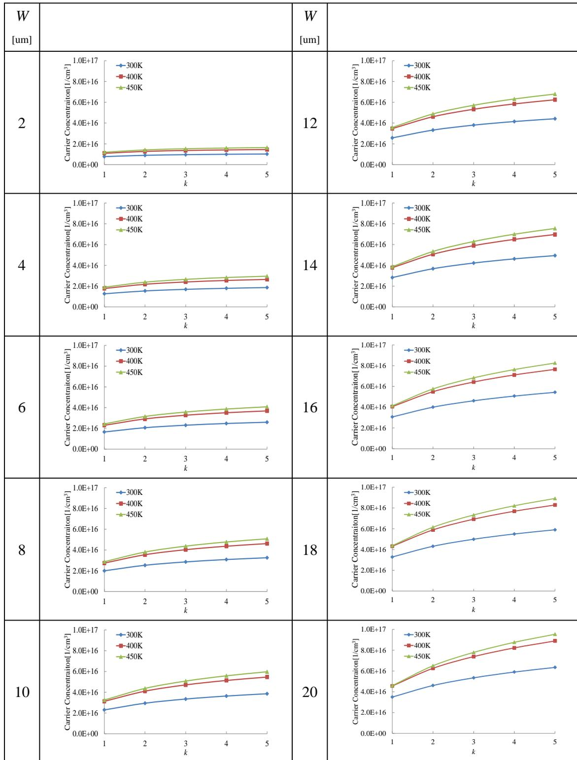
Figure 82. Relationships between carrier concentration and scaling factor  $k$ . Higher temperature makes higher injection efficiency especially with large  $k$ . The electron injection efficiency is assumed as 0.75.
