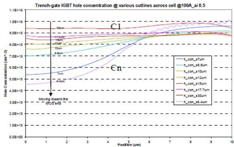
Fig. 6 Carrier concentration along horizontal cutlines C1, C2... Cn defined in Fig. 4.
