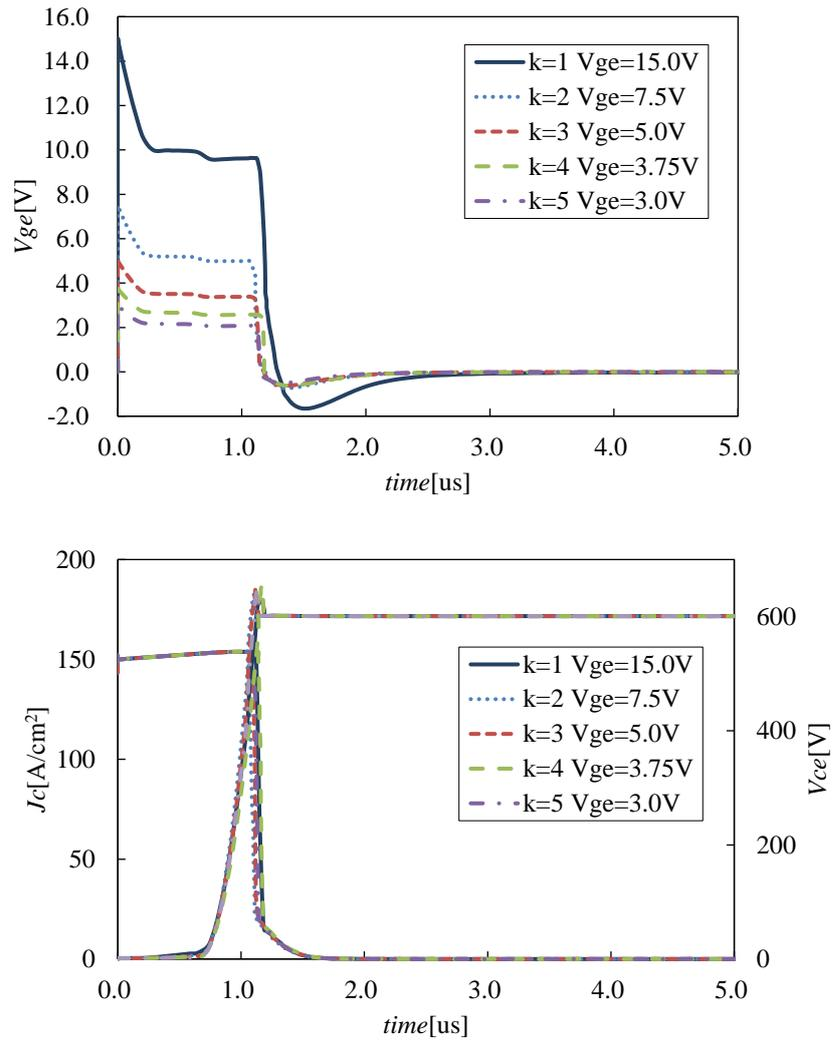
Figure 73. Calculated Turn-off characteristics of scaled devices with  $V_{th}$  adjustment. Device active area is  $1\text{cm}^2$ . Applied gate voltage is scaled by keeping constant electric field in gate oxide as  $E_{ox}'=E_{ox}$ . All devices show almost same turn-off characteristics by  $V_{th}$  adjustment.
