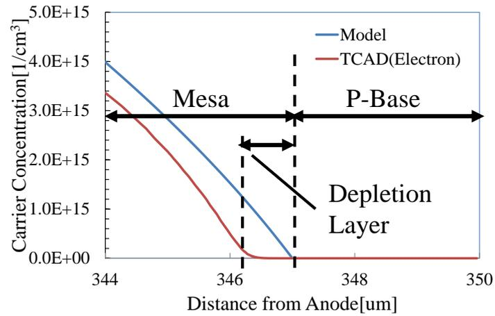
Figure 46. Carrier distribution in mesa region of 3.3kV IEGT at 50A/cm<sup>2</sup>.
