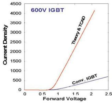
Fig.3 V-I curve comparison between proposed theory, TCAD result and conventional 600V IGBTs. (Theory and TCAD exactly coincides with each other) ( $a=3.7e18$ ,  $b=9.39e16$ )
