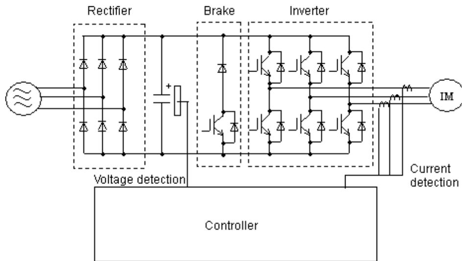
Figure 2. Motor control circuit example [2]. Six IGBT chips on “Inverter” bridge convert to three phase AC power with arbitrary frequency and voltage.
