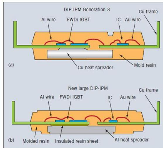
Fig. 1. Cross-sections of the a) previous Generation 3 DIP-IPM and b) the new Generation 4 DIP-IPM.
