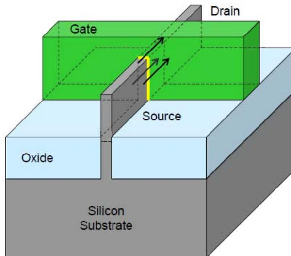
Figure 86. Latest transistor cell in 2012 [52]. Three dimensional structure, called “Tri-Gate”, is used to prevent off-state leakage current, keeping enough on-state current level.
