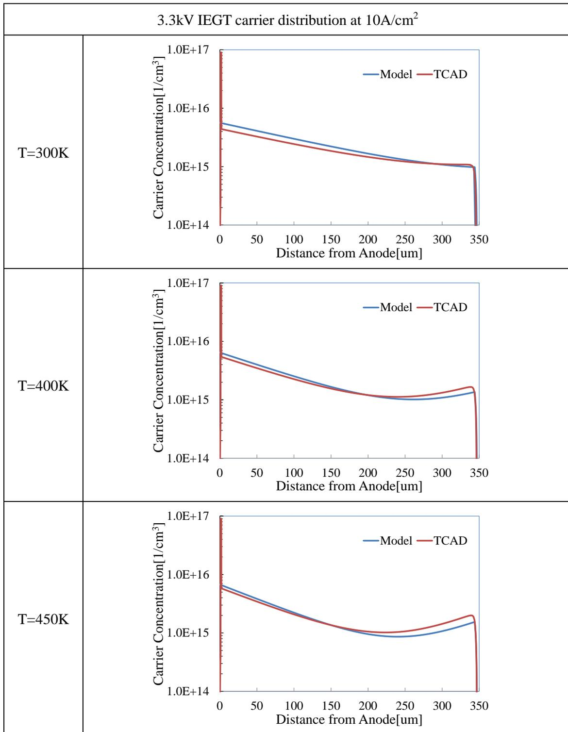
Figure 38. Calculated carrier distribution comparison between proposed compact model and TCAD simulator for 3.3kV IEGT at  $10\text{A}/\text{cm}^2$ .
