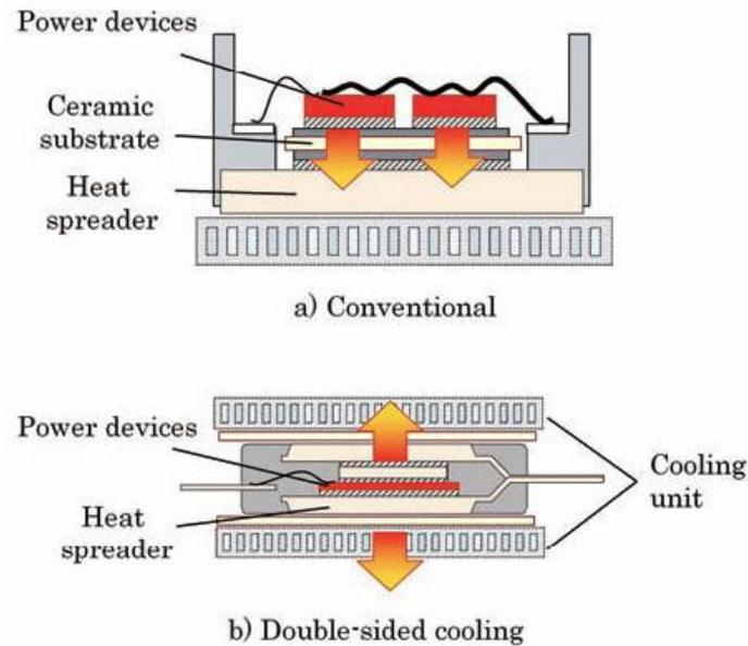
Fig. 3 Cross sectional view of a conventional power module and a double sided power module
