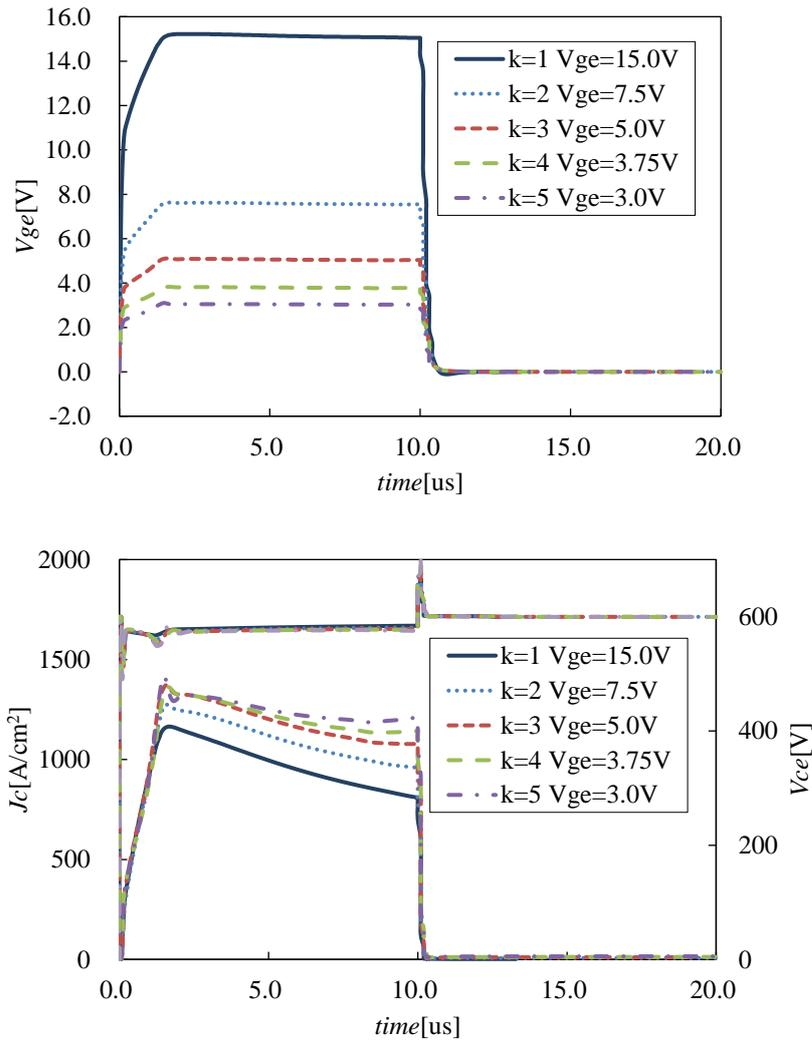
Figure 74. Calculated short-circuit waveforms of scaled devices with  $V_{th}$  adjustment. Applied gate voltage is scaled by keeping constant electric field in gate oxide as  $E_{ox} = E_{ox}$ . Lower and similar saturation current are realized. No thermal runaway was occurred.
