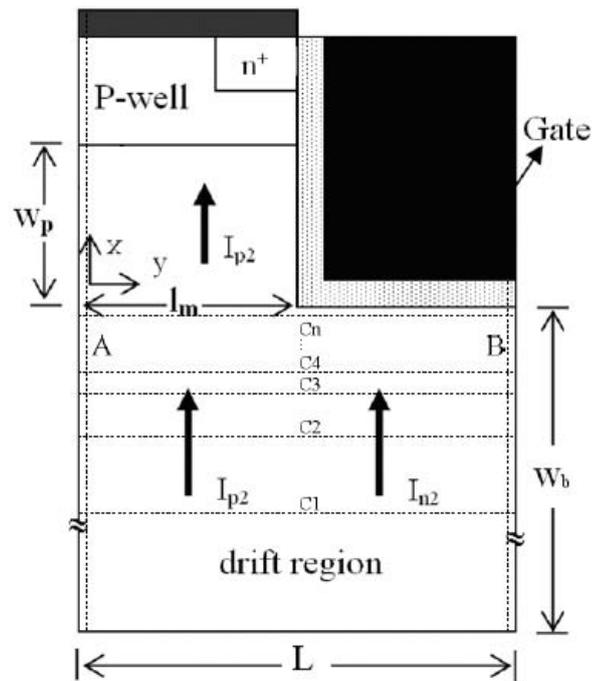
Fig. 4 Trench IGBT structure with physical dimensions. Vertical cutlines A, B and horizontal cutlines C1, C2... Cn are also shown.
