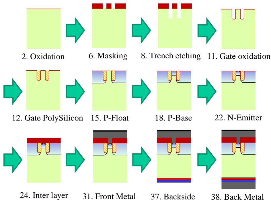
Figure 76. An example of “cell first” process flow.
