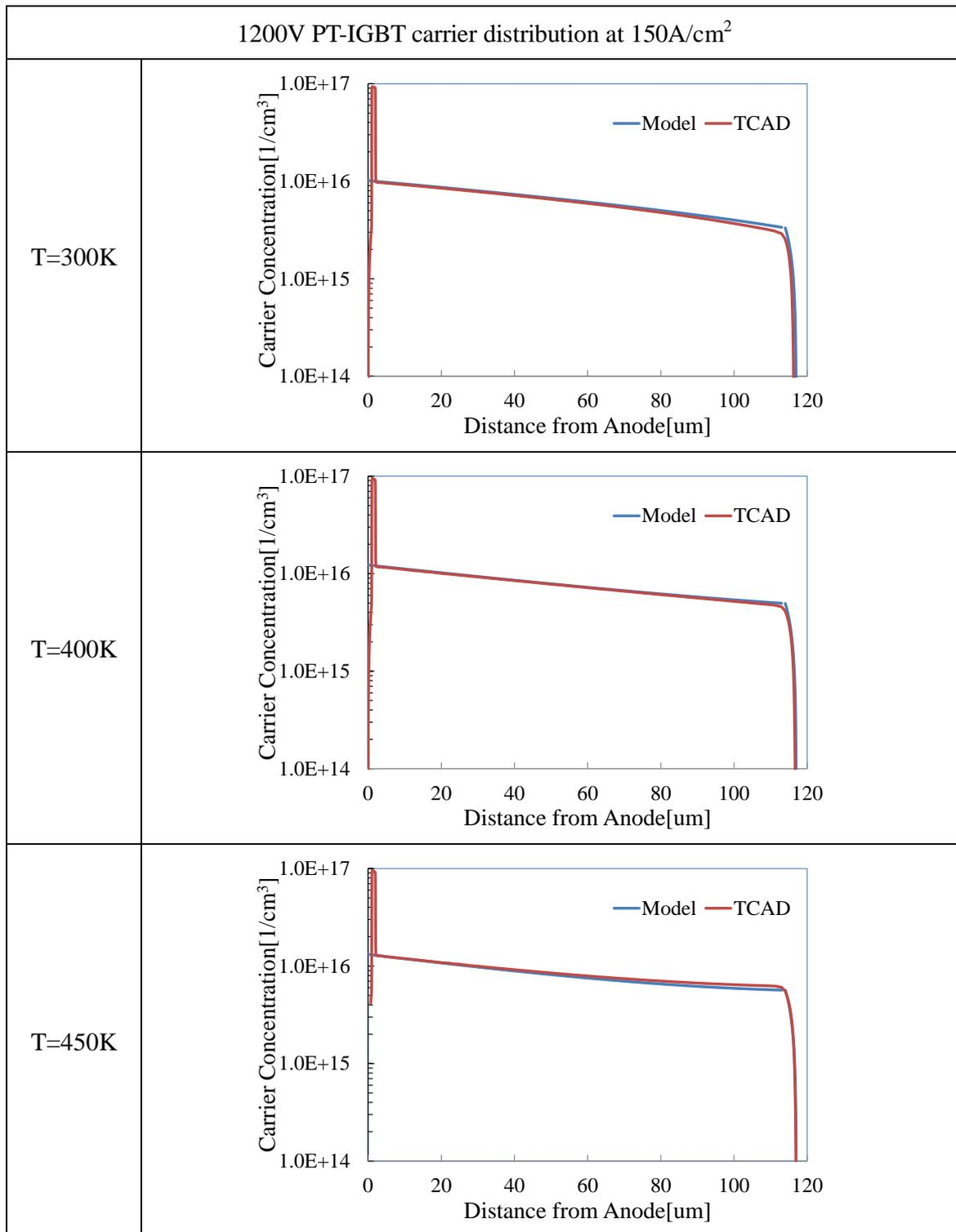
Figure 36. Calculated carrier distribution comparison between proposed compact model and TCAD simulator for 1200V PT-IGBT at 150A/cm<sup>2</sup>.
