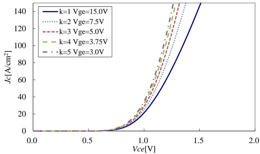
Figure 72. Calculated  $I_c$ - $V_c$  characteristics of scaled devices with  $V_{th}$  adjustment and constant electric field in gate oxide as  $E_{ox}' = E_{ox}$ .  $V_{ce(sat)}$  is improved by increasing scaling factor  $k$ .
