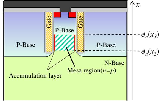
Figure 13. The main idea of the model. Current flow paths are assumed to accumulation layer and mesa region.
