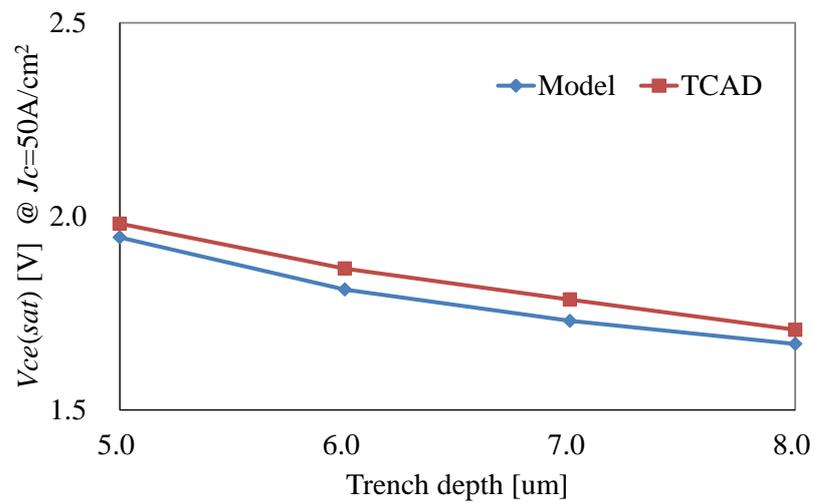
Figure 41. Trench depth- $V_{ce(sat)}$  relationship comparison between proposed model and TCAD for 3.3kV IEGT.
