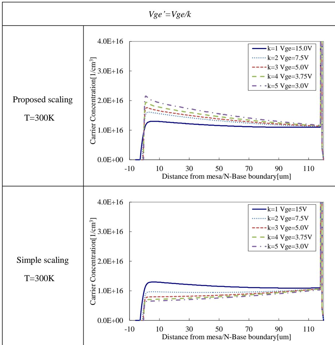
Figure 67. Calculated carrier distribution in N-Base region for scaling factor  $k=1$  to 5. The zero point of horizontal scale is set to mesa/N-Base boundary. In proposed scaling, Cathode side carrier concentration is increased by scale down. In simple scaling, Cathode side carrier concentration becomes lower with increasing scaling factor  $k$ .
