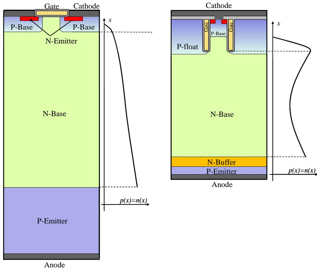
Figure 10. Carrier distribution for conduction mode. Electron and hole form same distribution in N-Base region. The left side figure shows Planar gate IGBT. The right side figure shows Trench gate IGBT. Carrier distribution profile is different.
