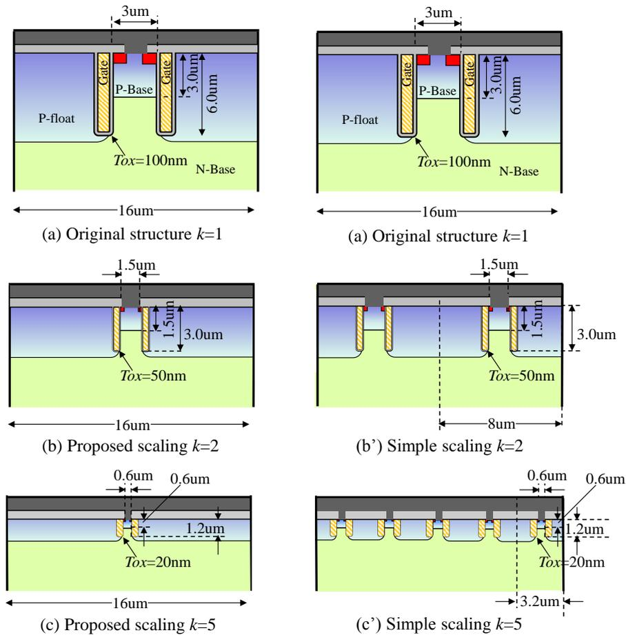
Figure 60. Proposed scaling (Left side) and Simple scaling (Right side). In proposed scaling, cell pitch is constant. In simple scaling, cell pitch is also scaled.
