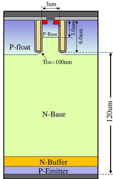
Figure 61. Base structure for scaling principle verification. 1200V PT-IGBT structure is used for the motif.
