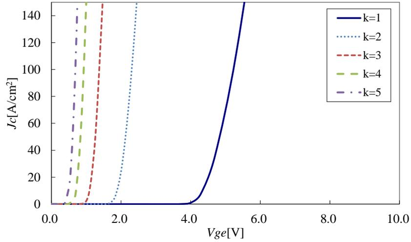
Figure 62.  $I_c$ - $V_{ge}$  characteristics for scaled devices. Scaled devices show lower  $V_{th}$  and higher  $g_m$ .
