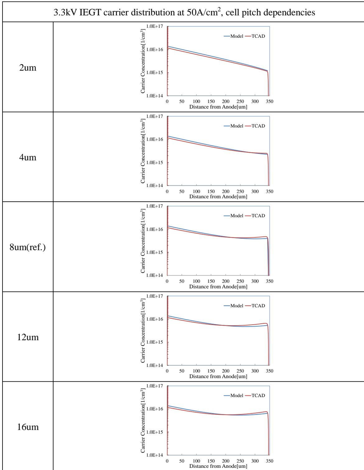
Figure 44. On-state carrier distribution profiles with varied half cell pitch for 3.3kV IEGT at  $50\text{A}/\text{cm}^2$ . Electron injection efficiency from Cathode side depends on the cell pitch.
