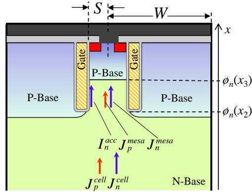
Figure 14. Current elements in Trench structure
