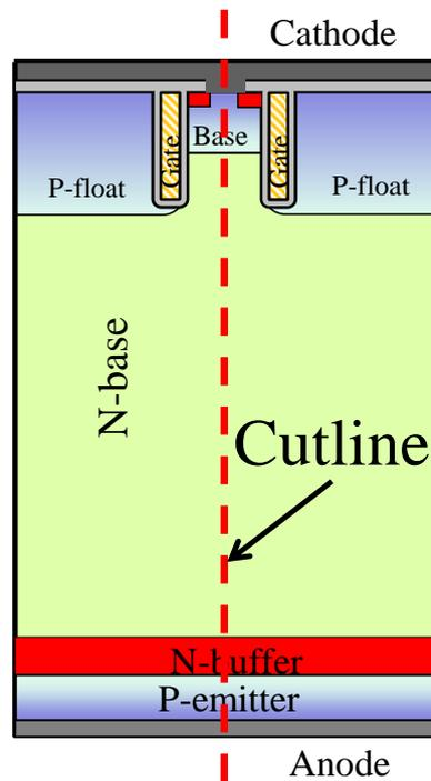
Figure 27. Carrier distribution profile measurement.
