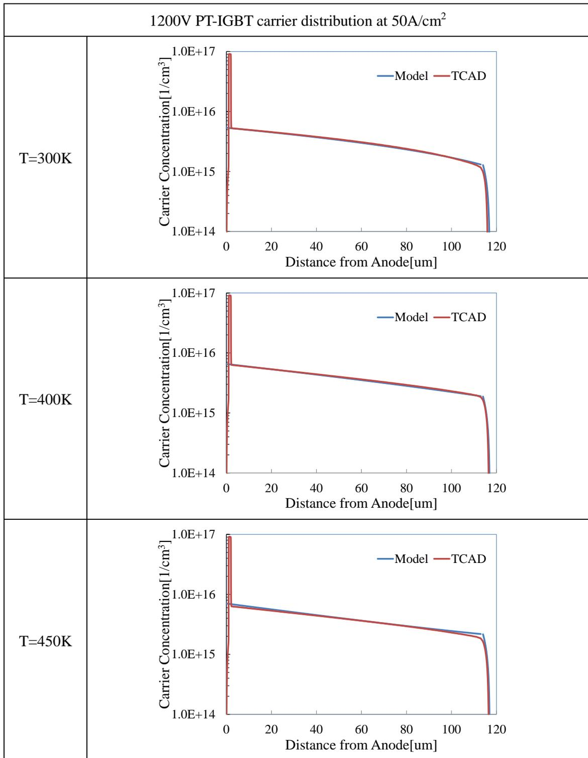
Figure 34. Calculated carrier distribution comparison between proposed compact model and TCAD simulator for 1200V PT-IGBT at 50A/cm<sup>2</sup>.
