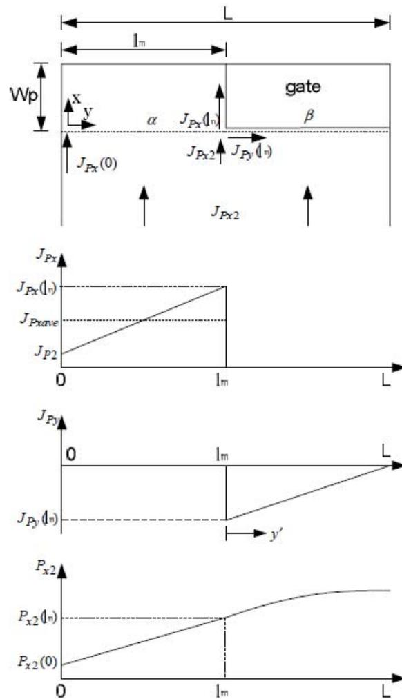
Fig. 17 From top to bottom: hole current flow at the MOS end, hole current density distributions  $J_{px}$  and  $J_{py}$  along cutlines  $\alpha$  and  $\beta$ , and carrier distribution along cutlines  $\alpha$  and  $\beta$ .
