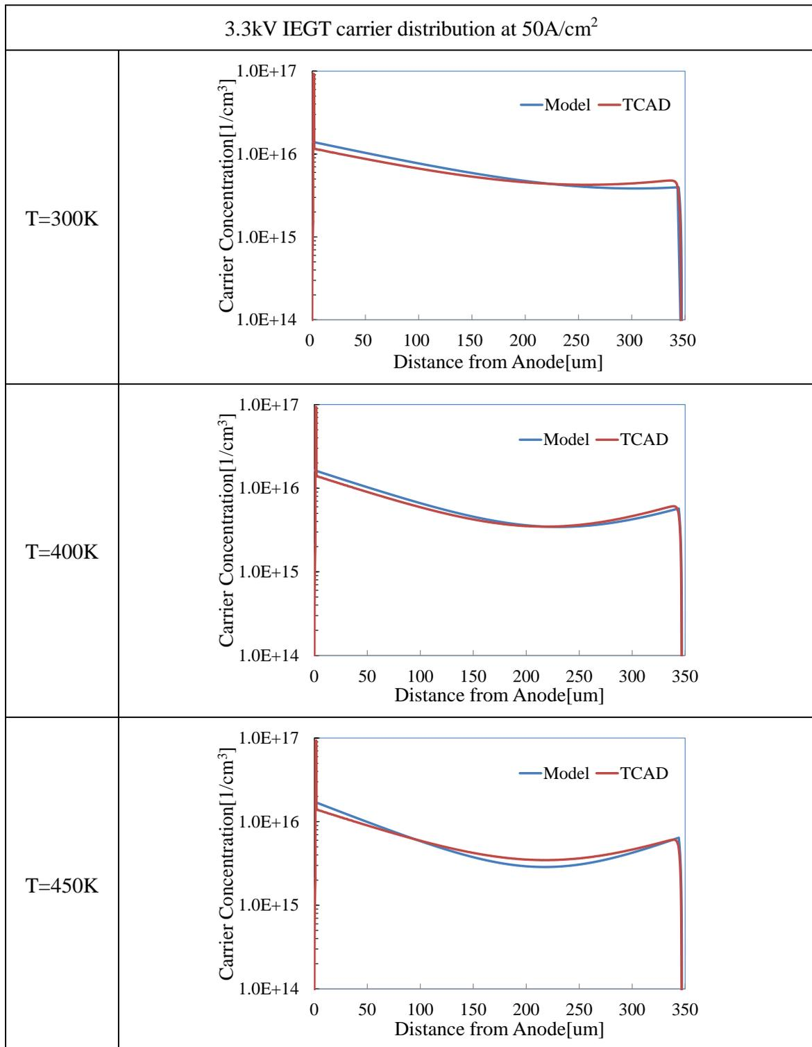
Figure 40. Calculated carrier distribution comparison between proposed compact model and TCAD simulator for 3.3kV IEGT at 50A/cm<sup>2</sup>.
