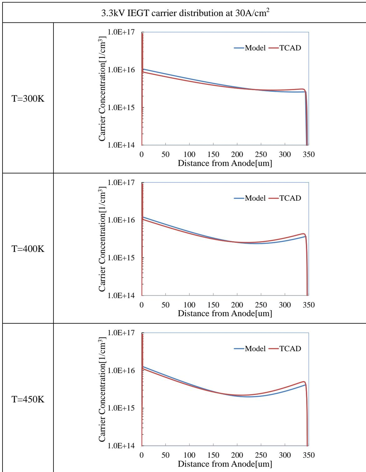
Figure 39. Calculated carrier distribution comparison between proposed compact model and TCAD simulator for 3.3kV IEGT at 30A/cm<sup>2</sup>.
