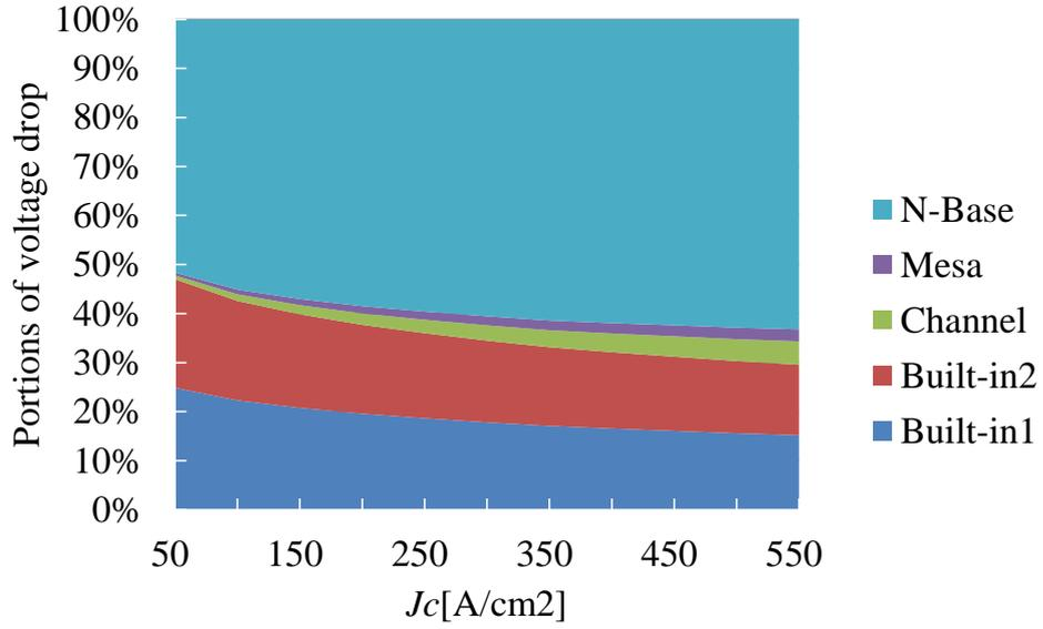
Figure 79. Portions of voltage drop at 300K for 1200V PT-IGBT calculated by the proposed compact model. N-Base voltage drop is dominant in high current density region.
