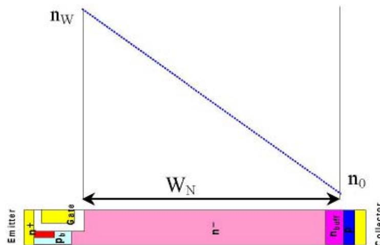
**Fig.1 Linearly graded carrier distribution in N-base**
