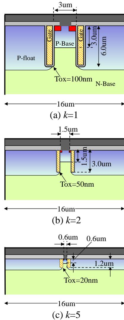
Figure 58. Proposed scaling principle for trench gate IGBT.
