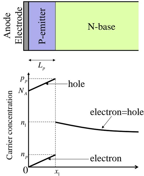
Figure 15. Structure and carrier distribution for NPT-IGBT with shallow P-Emitter
