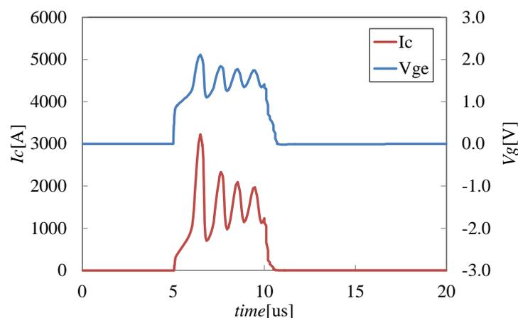
Figure 90. Oscillation waveform during short circuit for scaled device of  $k=5$ . Applied gate voltage=1.5V. Collector current oscillation is caused by the gate voltage.
