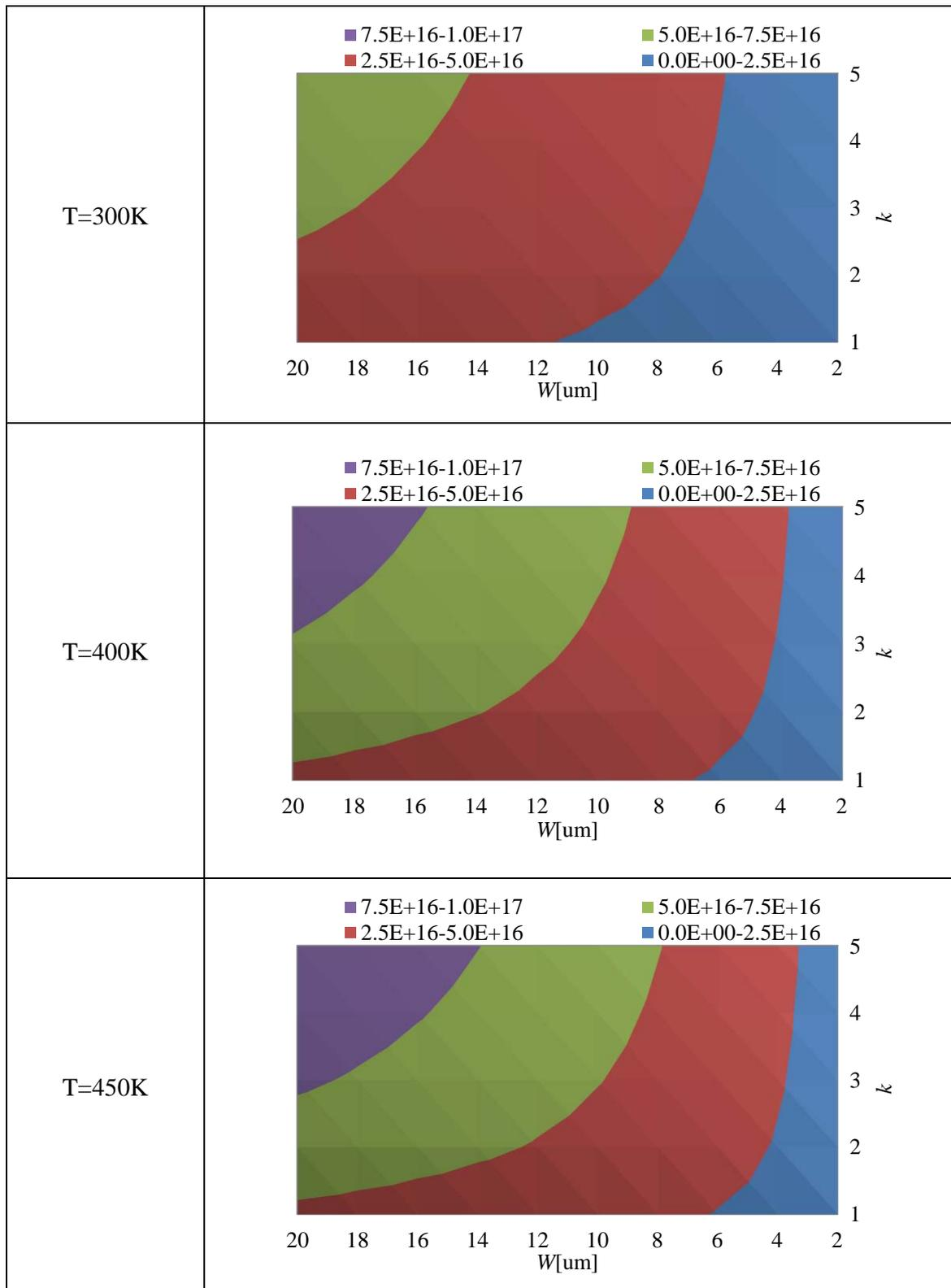
Figure 81. Relationship between cell pitch  $W$ , scaling factor  $k$  and carrier concentration  $n$  at N-Base/mesa boundary for  $450\text{A}/\text{cm}^2$ . The electron injection efficiency is assumed as 0.75.
