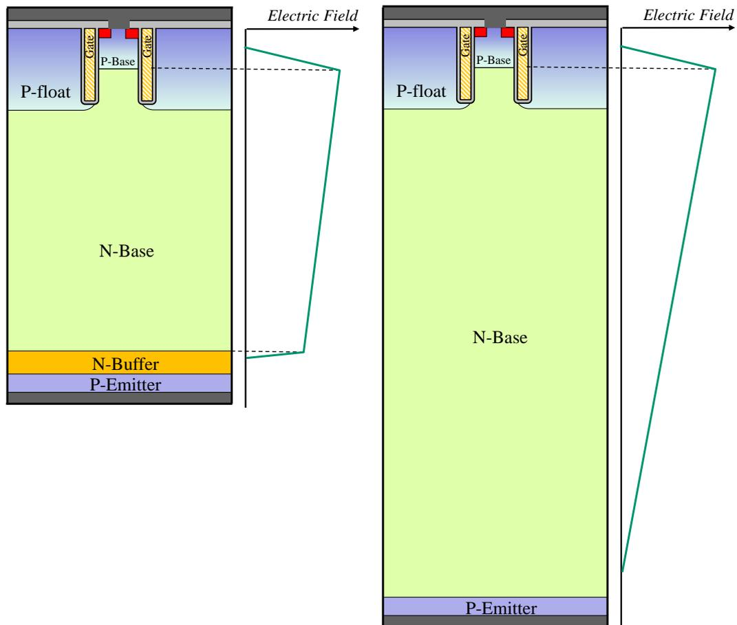
Figure 11. Electric field distribution in off state (left: PT-IGBT, right: NPT-IGBT).
