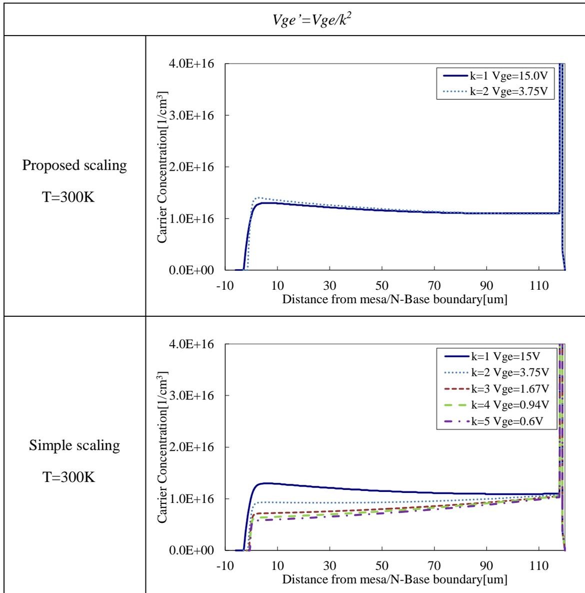
Figure 64. Calculated carrier distribution in N-Base region of scaled devices with scaled electric field in gate oxide as  $E_{ox}' = E_{ox}/k$ . The zero point of horizontal scale is set to mesa/N-Base boundary. In proposed scaling, similar carrier distribution is obtained instead of scale down. In simple scaling, Cathode side carrier concentration becomes lower with increasing scaling factor  $k$ .
