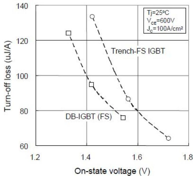
Figure 3. Simulated trade-off relationship between  $V_{ON}$  and  $E_{OFF}$  of the DB-IGBT and the trench IGBT with FS backside structure
