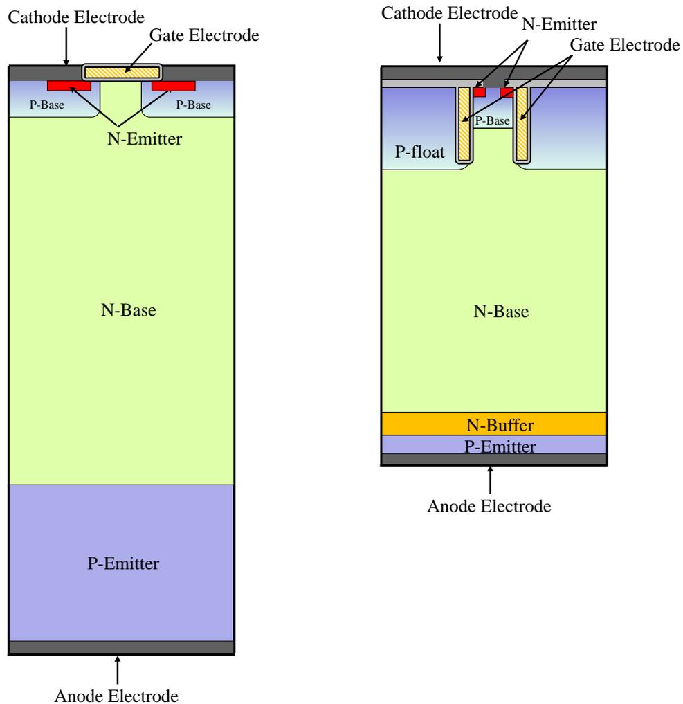
Figure 9. IGBT structure. The left side figure shows old designed Planar gate thick wafer IGBT. The right side figure shows newest Trench gate thin wafer IGBT.
