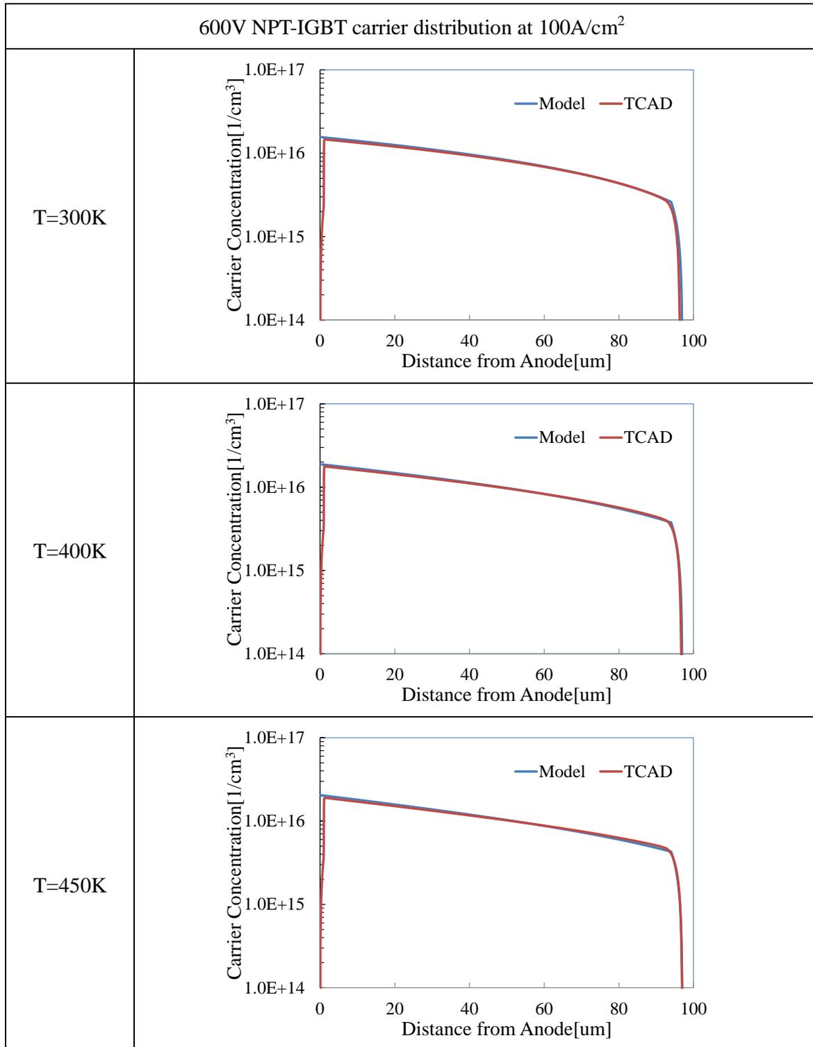
Figure 30. Calculated carrier distribution comparison between proposed compact model and TCAD simulator for 600V NPT-IGBT at 100A/cm<sup>2</sup>.
