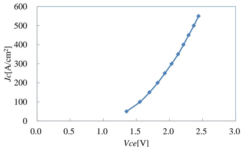
Figure 78.  $I_c$ - $V_{ce}$  characteristic for 1200V PT-IGBT calculated by the proposed compact model. To improve power density,  $V_{ce}(sat)$  must be reduced in high current density region.
