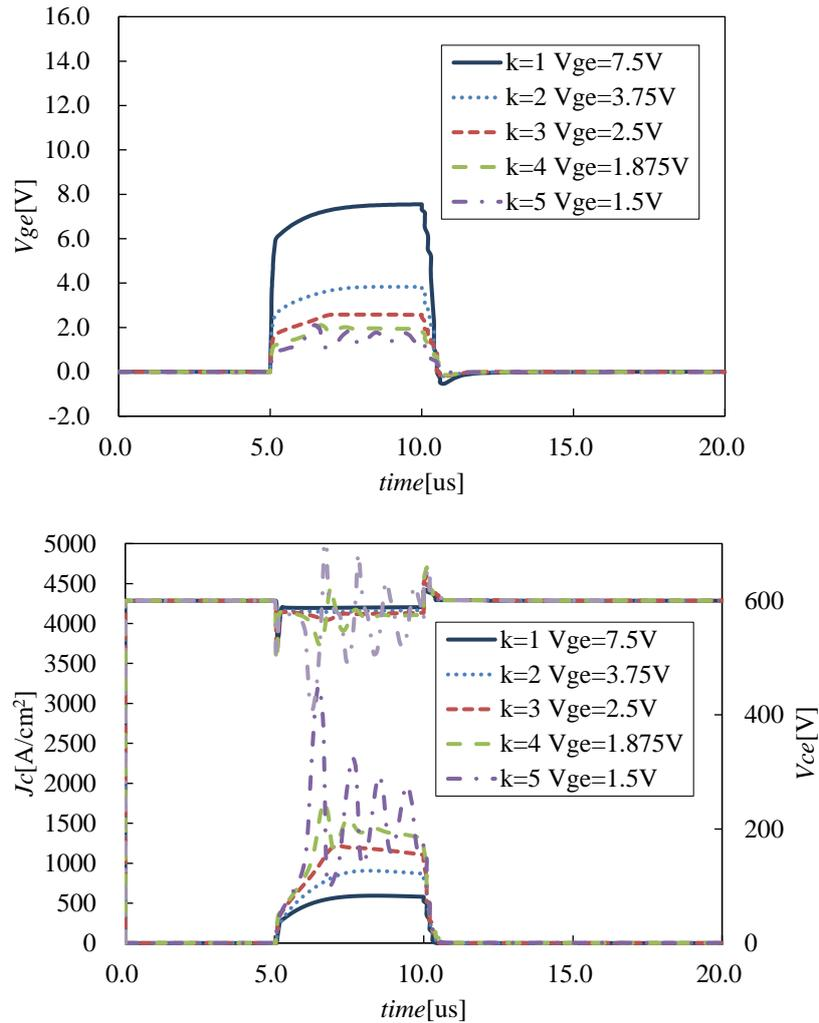
Figure 70. Calculated short-circuit waveforms of proposed scaling devices with constant electric field in gate oxide as  $E_{ox}'=E_{ox}$ . Lower gate voltage was applied to avoid thermal runaway in this calculation.
