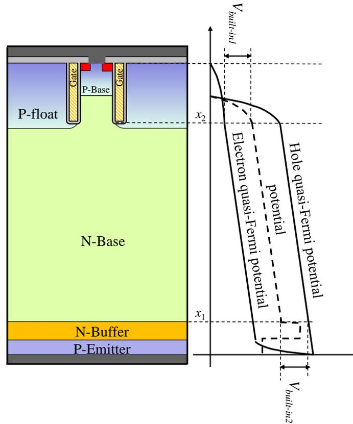
Figure 24. Built-in potential definition for the model.
