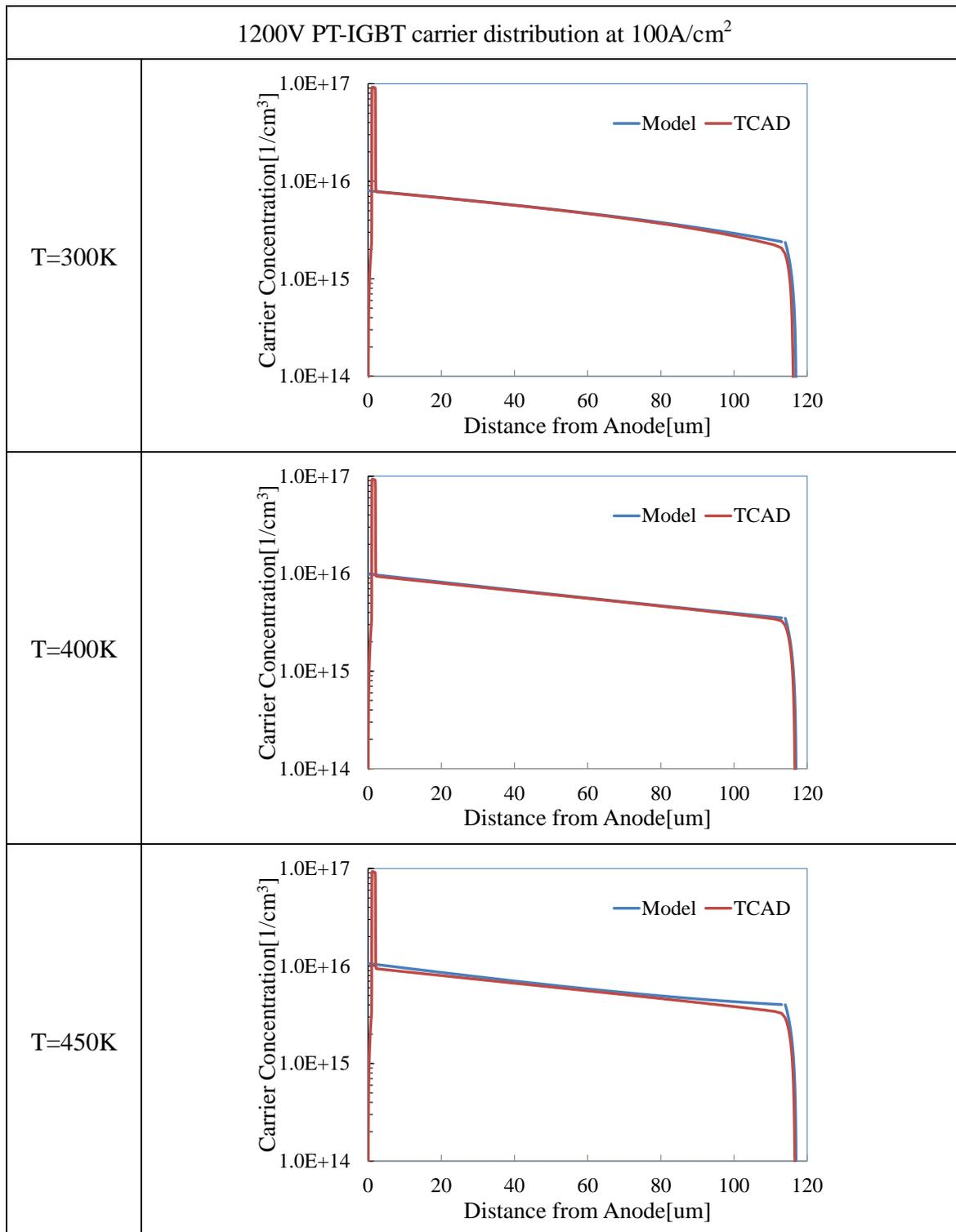
Figure 35. Calculated carrier distribution comparison between proposed compact model and TCAD simulator for 1200V PT-IGBT at 100A/cm<sup>2</sup>.
