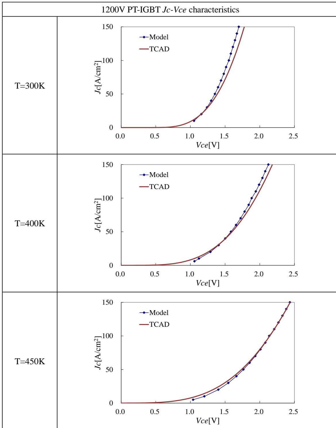
Figure 33. Calculated  $J_c$ - $V_{ce}$  characteristic comparison between proposed compact model and TCAD simulator for 1200V PT-IGBT.
