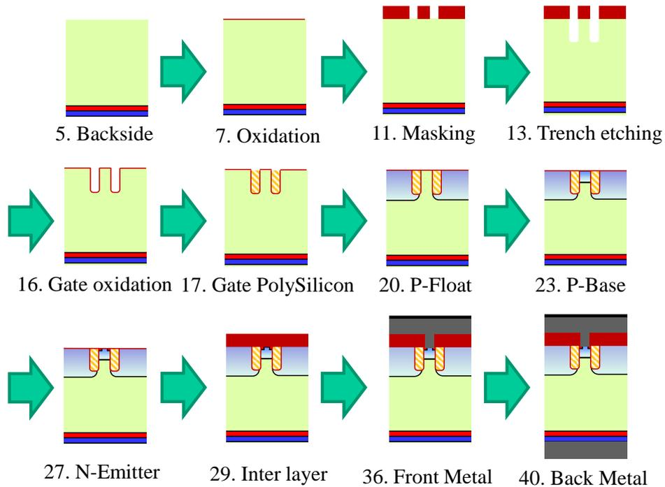
Figure 77. An example of “cell last” process flow.
