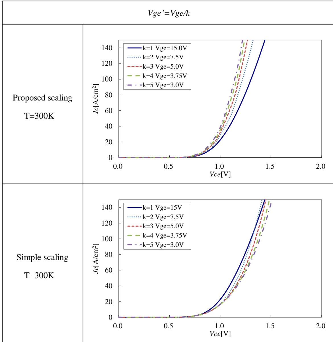
Figure 65. Calculated  $I_c$ - $V_c$  characteristics of scaled devices with constant electric field in gate oxide as  $E_{ox}' = E_{ox}$ . In proposed scaling,  $V_{ce}(sat)$  is improved by increasing scaling factor  $k$ . In simple scaling,  $V_{ce}(sat)$  becomes higher with increasing scaling factor  $k$ .
