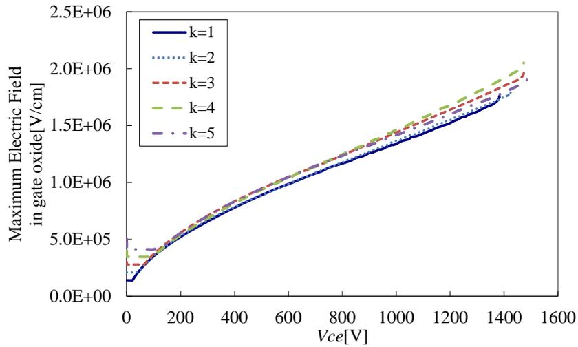
Figure 75. Simulated maximum electric field in gate oxide for static breakdown.
