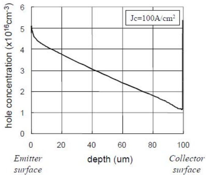
Figure 2. Simulated hole profile of the DB-IGBT under steady on-state
