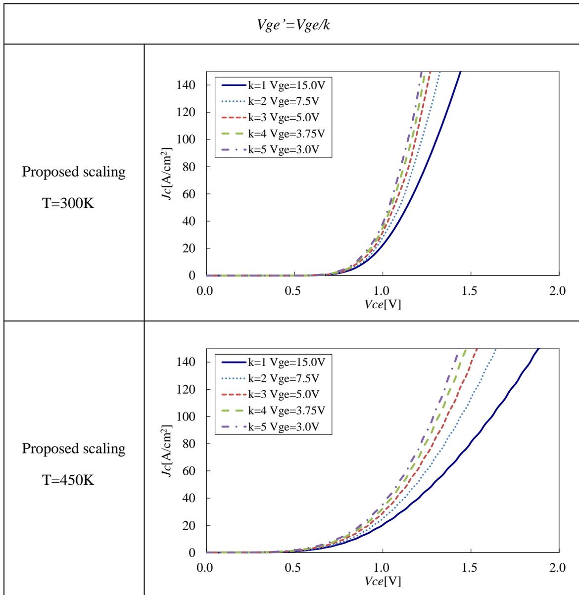
Figure 66. Calculated  $I_c$ - $V_c$  characteristics of proposed scaling devices with constant electric field in gate oxide as  $E_{ox}' = E_{ox}$ . In higher temperature condition,  $V_{ce}(sat)$  improved especially.
