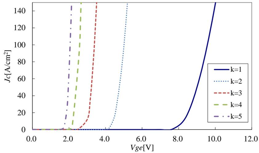
Figure 71.  $I_c$ - $V_{ge}$  characteristics for scaled devices with  $V_{th}$  adjustment. Scaled devices show higher  $g_m$ .
