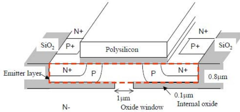
Figure 1. Schematic cross sectional view of a DB-IGBT
