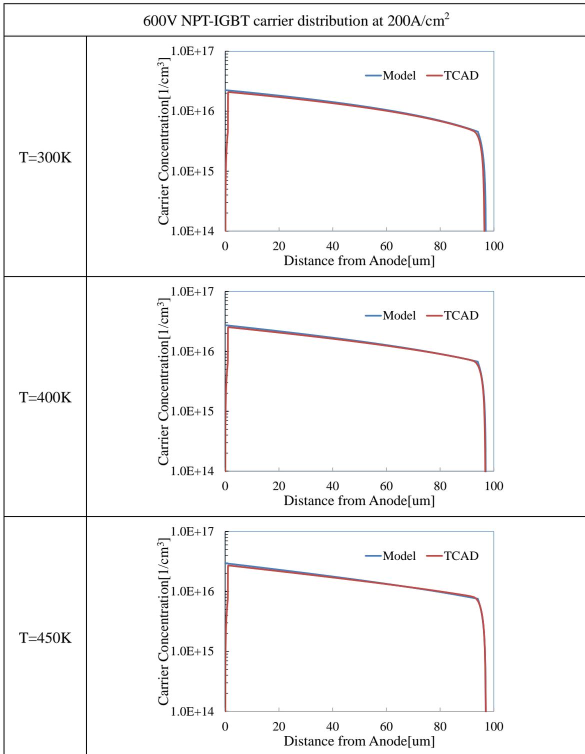
Figure 32. Calculated carrier distribution comparison between proposed compact model and TCAD simulator for 600V NPT-IGBT at 200A/cm<sup>2</sup>.
