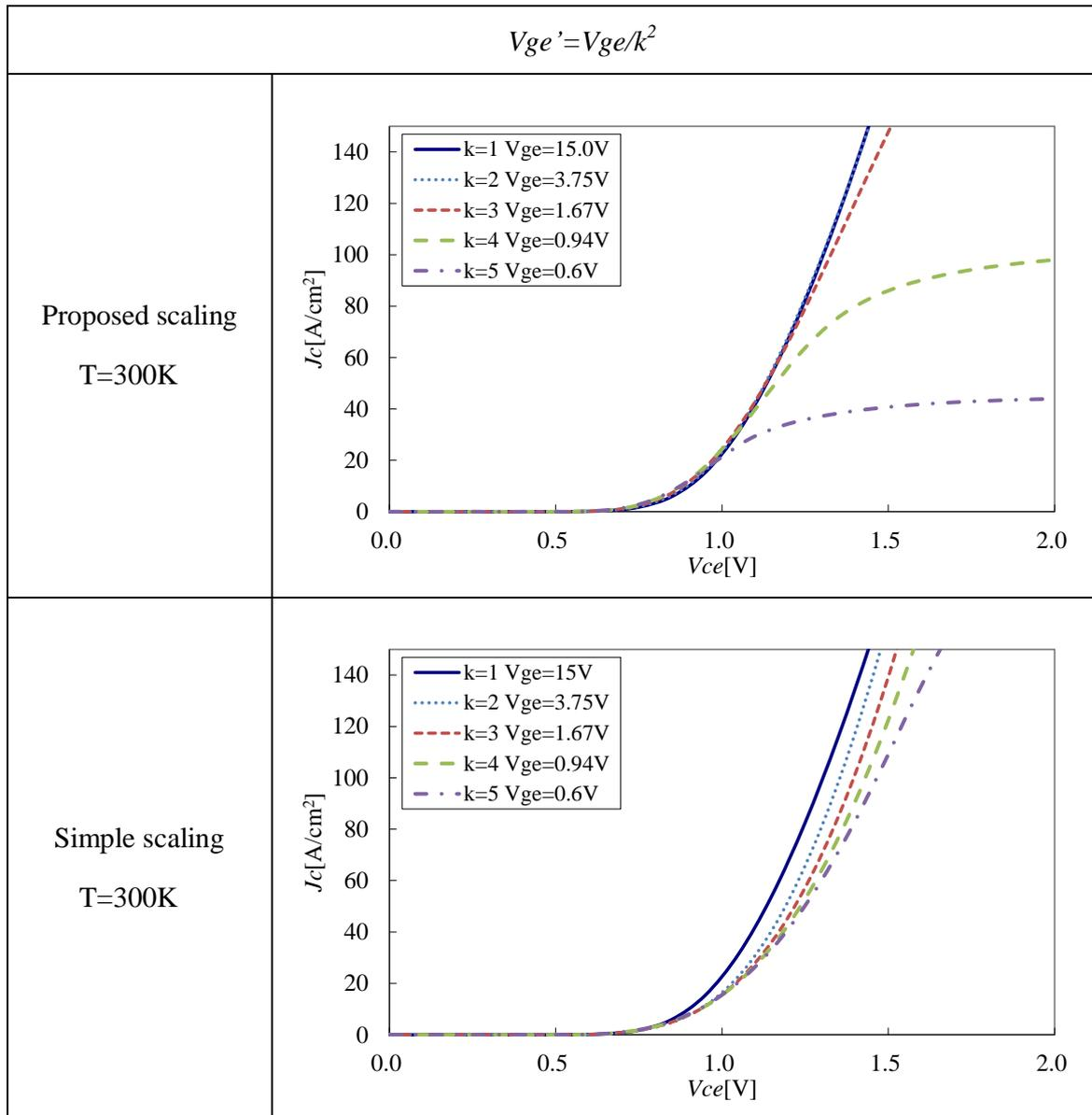
Figure 63. Calculated  $I_c$ - $V_c$  characteristics of scaled devices with scaled electric field in gate oxide as  $E_{ox}' = E_{ox}/k$ . In proposed scaling,  $k=1$  and 2 show good agreement but more scaled devices show lower saturation current. In simple scaling,  $V_{ce}(sat)$  becomes higher with increasing scaling factor  $k$ .
