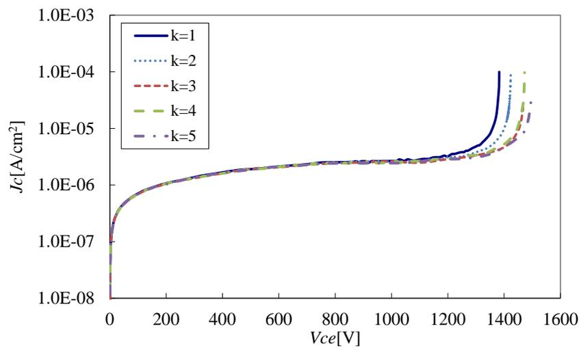
Figure 83. Breakdown characteristics for scaled devices.
