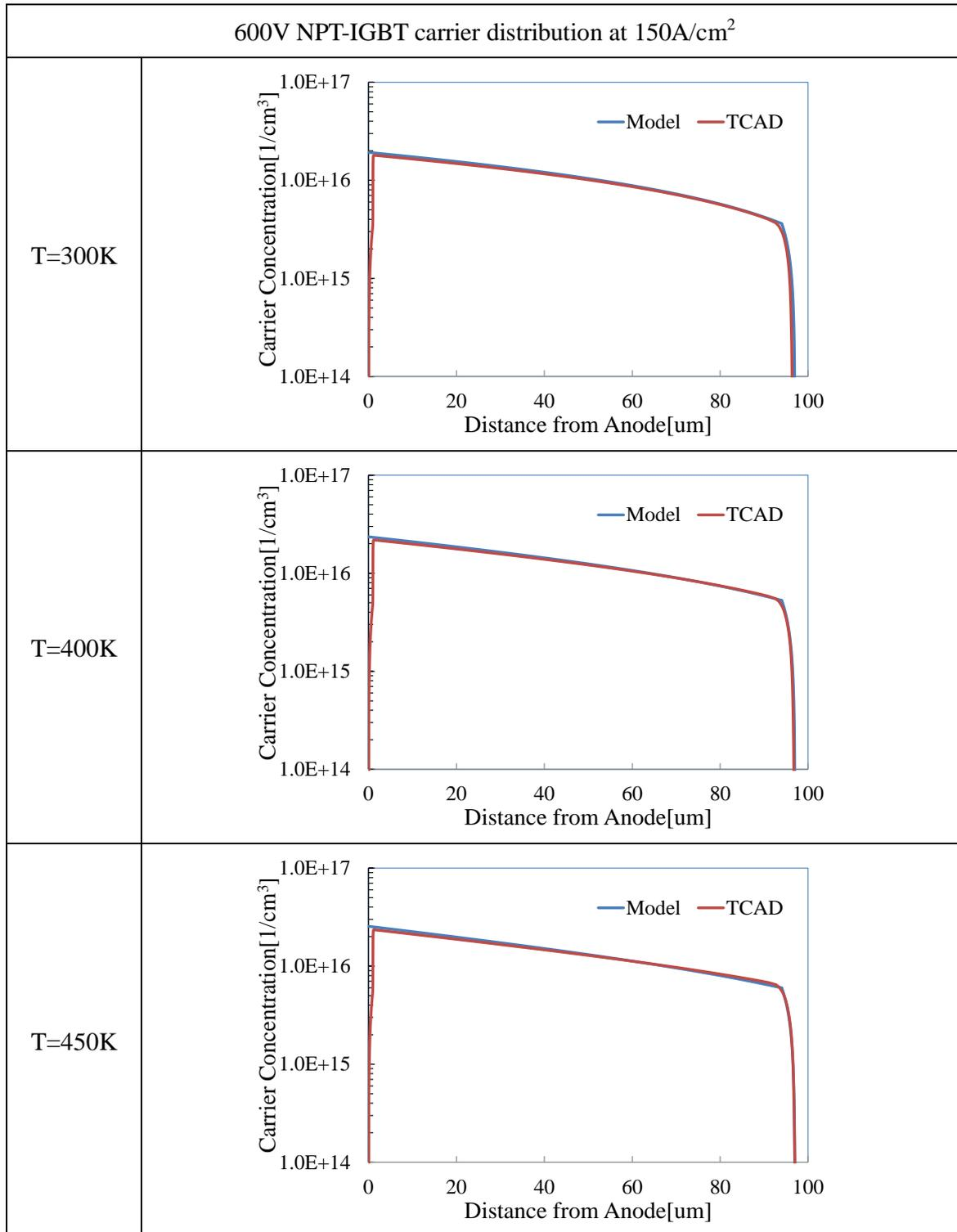
Figure 31. Calculated carrier distribution comparison between proposed compact model and TCAD simulator for 600V NPT-IGBT at 150A/cm<sup>2</sup>.
