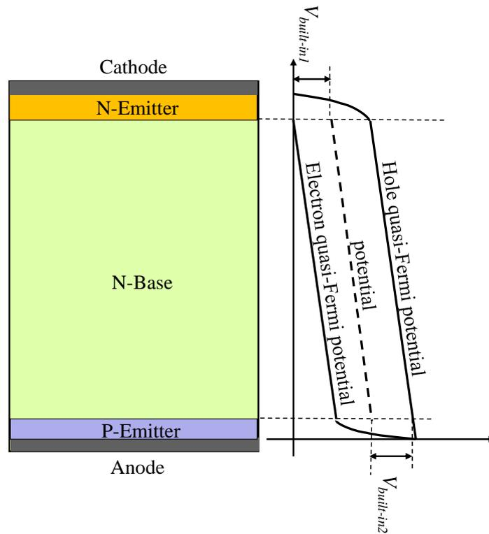
Figure 23. Built-in potential for high injection devices.
