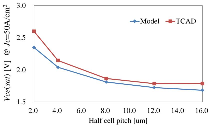
Figure 42. Cell pitch- $V_{ce(sat)}$  relationship comparison between proposed model and TCAD for 3.3kV IEGT.
