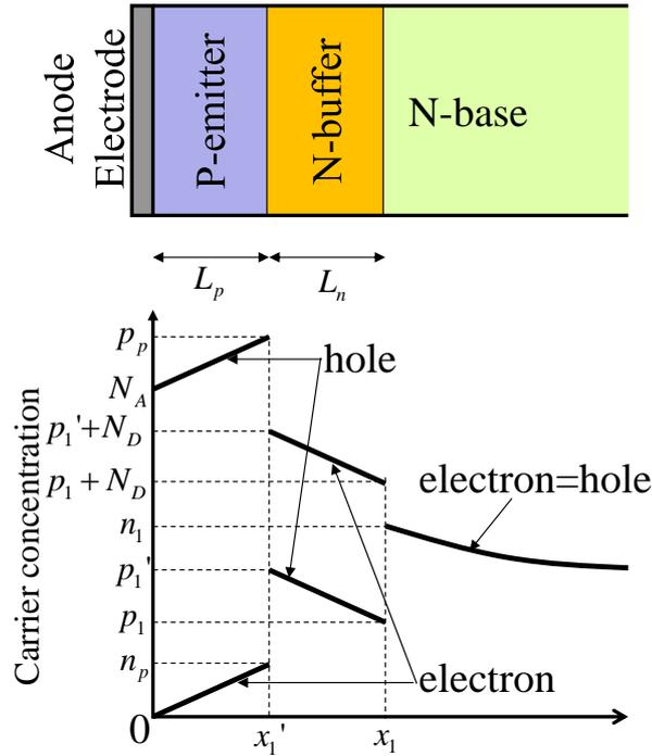
Figure 16. Structure and carrier distribution for PT-IGBT with shallow P-Emitter and shallow N-Buffer
