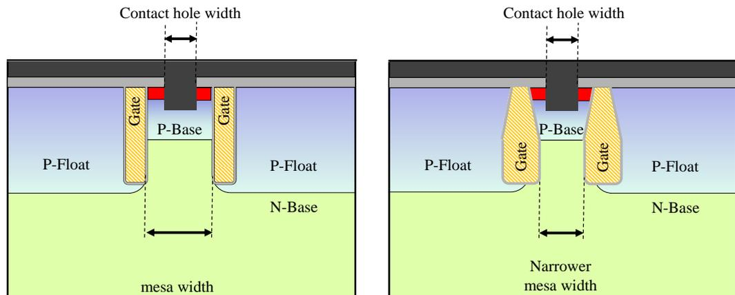
Figure 87. A structure to keep lower contact resistance and avoid electro migration (right side). Mesa width limitation is exist in conventional cell design (left side).
