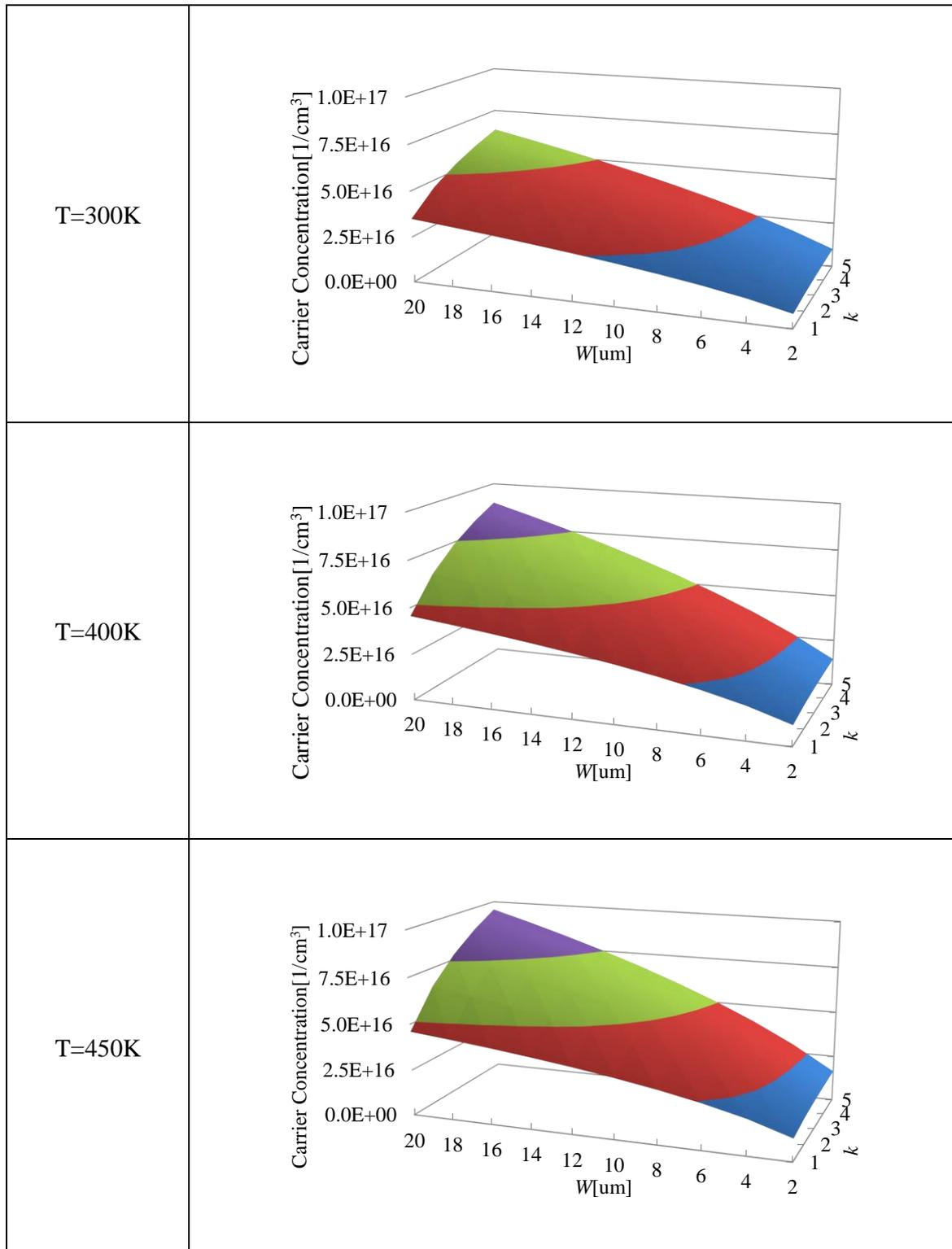
Figure 80. Relationship between cell pitch  $W$ , scaling factor  $k$  and carrier concentration  $n$  at N-Base/mesa boundary for  $450\text{A}/\text{cm}^2$ . The electron injection efficiency is assumed as 0.75.
