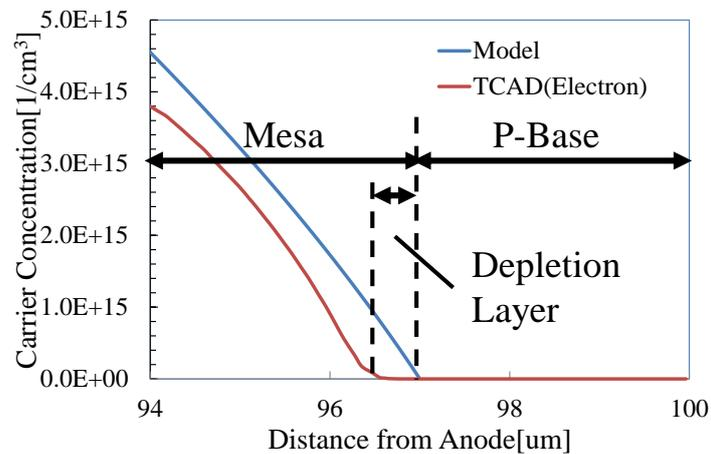
Figure 45. Carrier distribution in mesa region of 600V NPT-IGBT at 200A/cm<sup>2</sup>.
