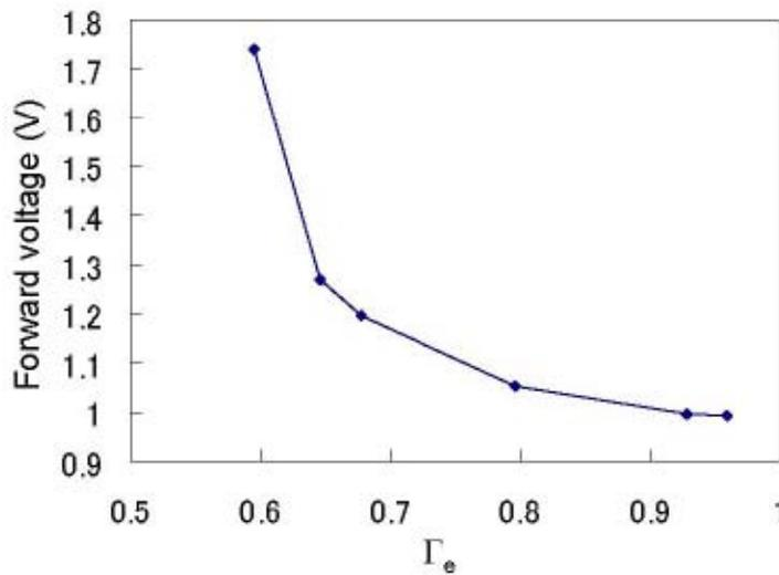
Fig.7 Forward voltage of 600V IGBTs at 500A/cm<sup>2</sup> as a function of electron injection efficiency,  $\Gamma_e$ .  $\Gamma_e$  of more than 0.8 is desired.
