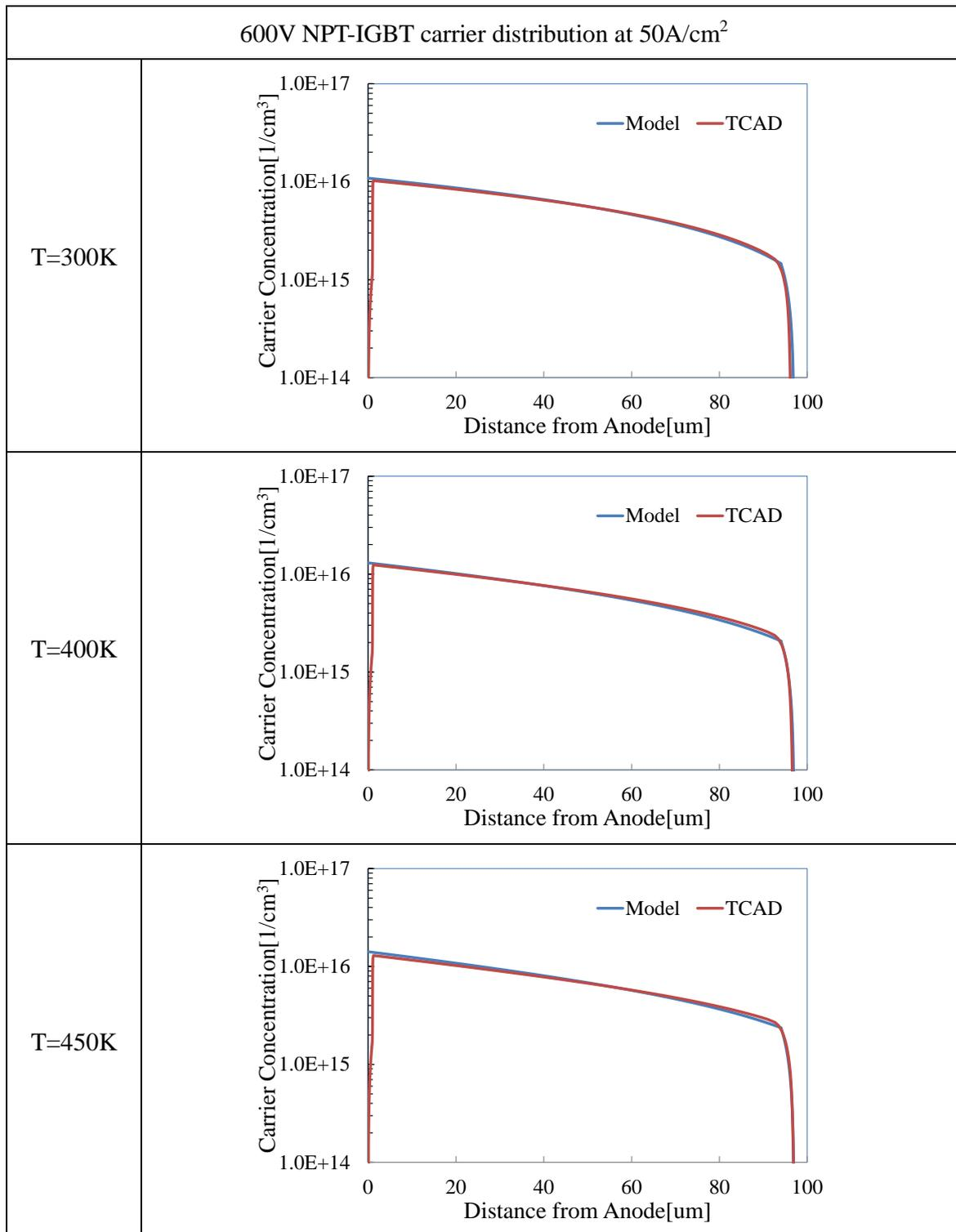
Figure 29. Calculated carrier distribution comparison between proposed compact model and TCAD simulator for 600V NPT-IGBT at 50A/cm<sup>2</sup>.
