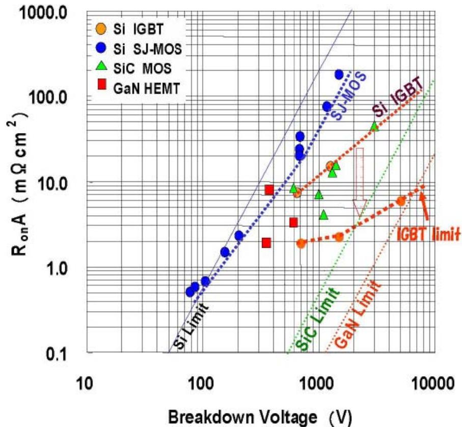
Fig.11 The proposed IGBT, denoted as “IGBT limit,” is compared with state of the art devices. Predicted IGBT limit surpasses so called SiC limit for over 2kV range.
