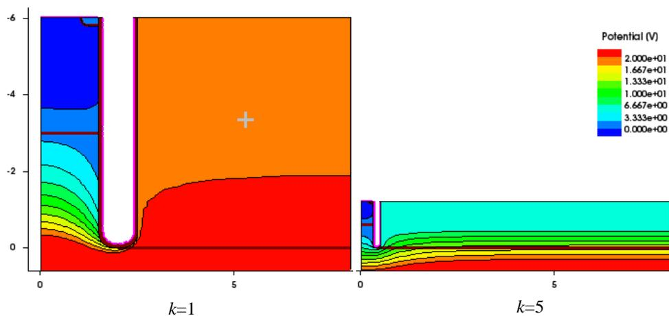
Figure 84. Potential distribution comparison between original device ( $k=1$ ) and scaled device ( $k=5$ ) at breakdown.
