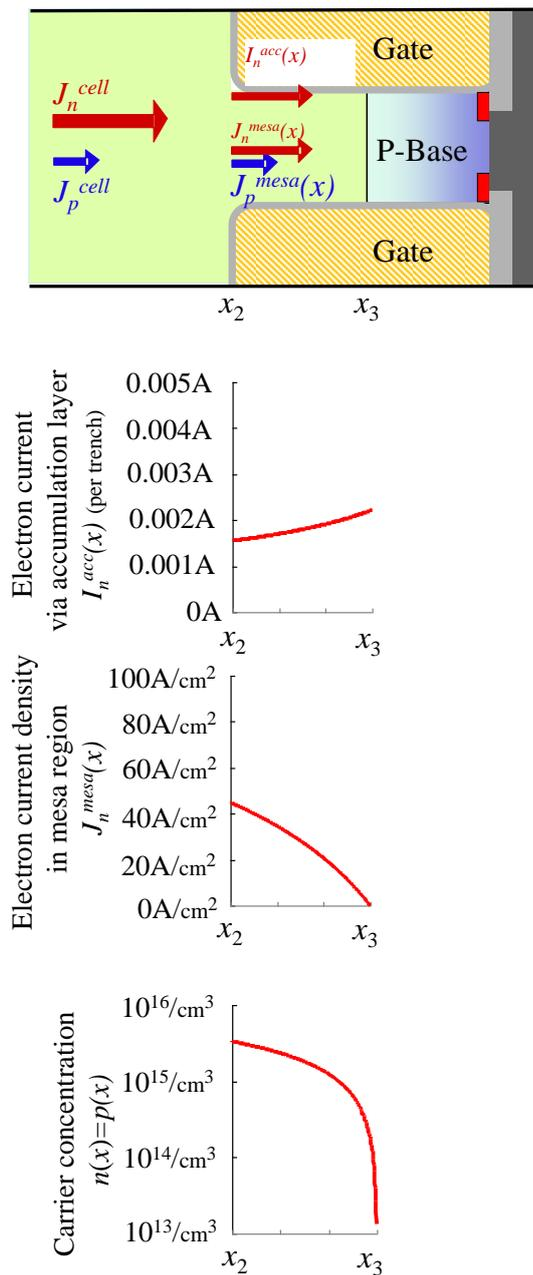
Figure 47. Relationship for carrier concentration in mesa region, electron current density in mesa region and electron current via accumulation layer. The structure is 1200V PT-IGBT. The current density is 150A/cm<sup>2</sup>.
