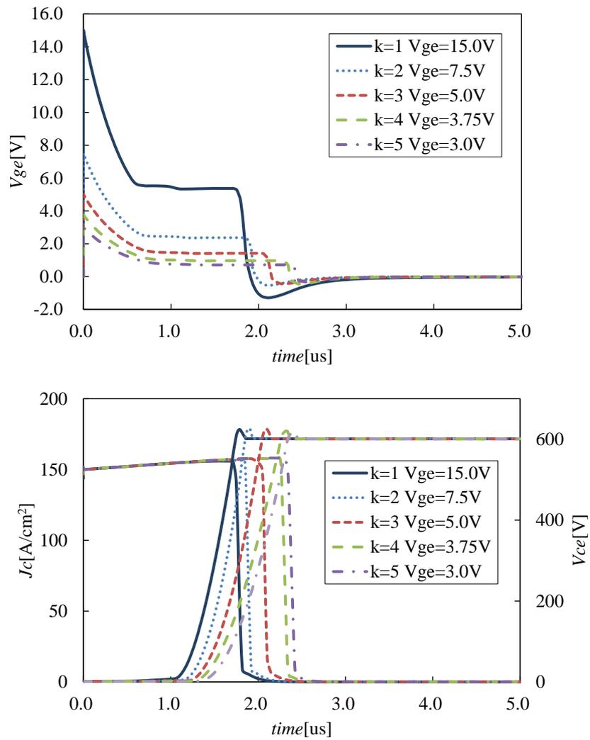
Figure 69. Calculated Turn-off characteristics of proposed scaling devices with constant electric field in gate oxide as  $E_{ox}'=E_{ox}$ . Device active area is  $1\text{cm}^2$ . Same external gate resistance of  $10\text{ohm}$  is used.
