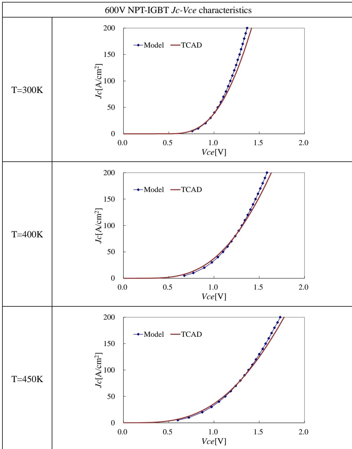
Figure 28. Calculated  $J_c$ - $V_{ce}$  characteristic comparison between proposed compact model and TCAD simulator for 600V NPT-IGBT.
