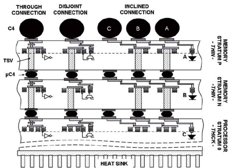
Figure 92. TSV (Through Silicon Via) technology [60].
