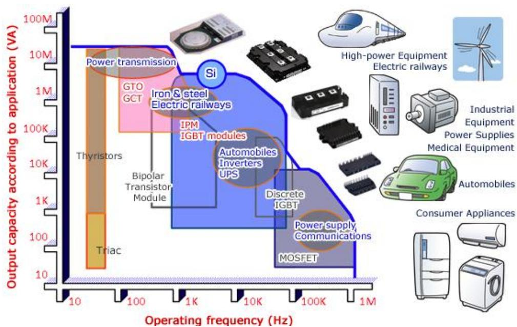
Figure 1. Cover area for various power devices [1].
