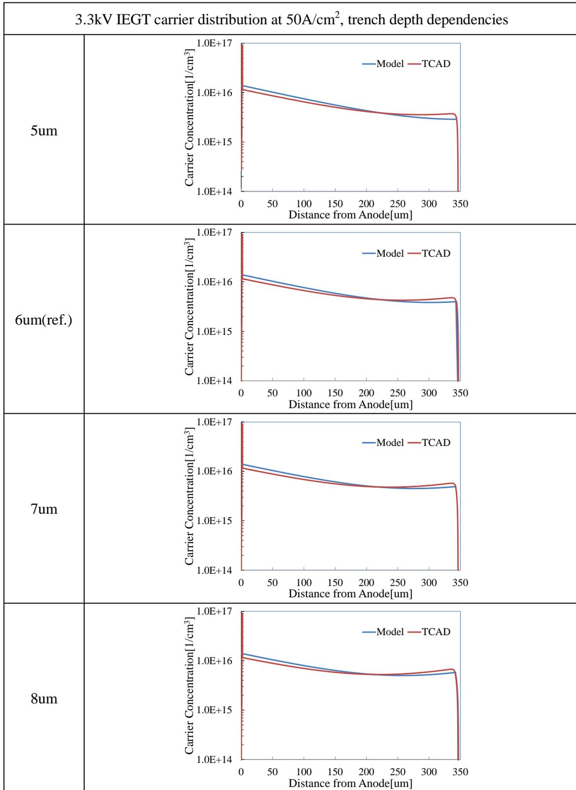
Figure 43. On-state carrier distribution profiles with varied trench depth for 3.3kV IEGT at 50A/cm<sup>2</sup>. Electron injection efficiency from Cathode side depends on the depth.
