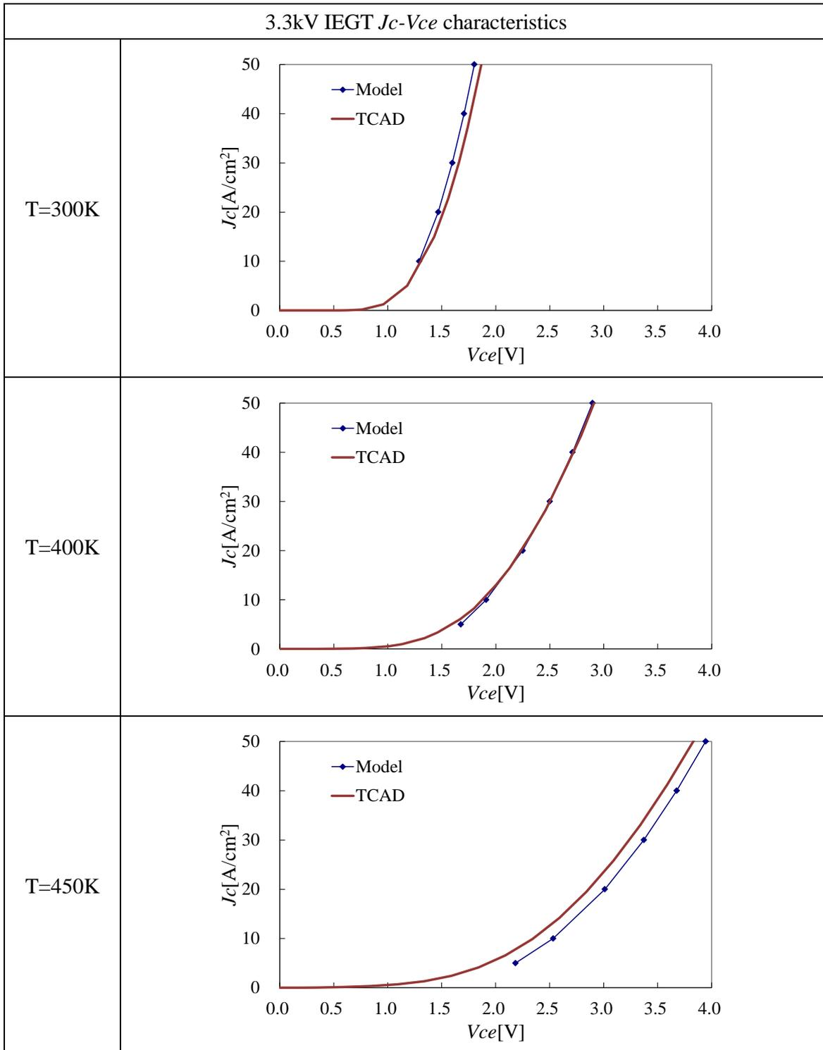
Figure 37. Calculated  $J_c$ - $V_{ce}$  characteristic comparison between proposed compact model and TCAD simulator for 3.3kV IEGT.
