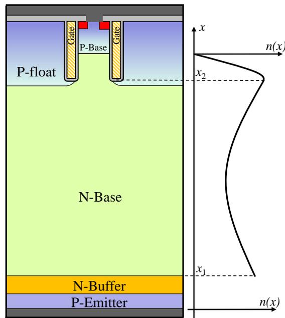
Figure 17 Cross sectional view of Trench gate IGBT
