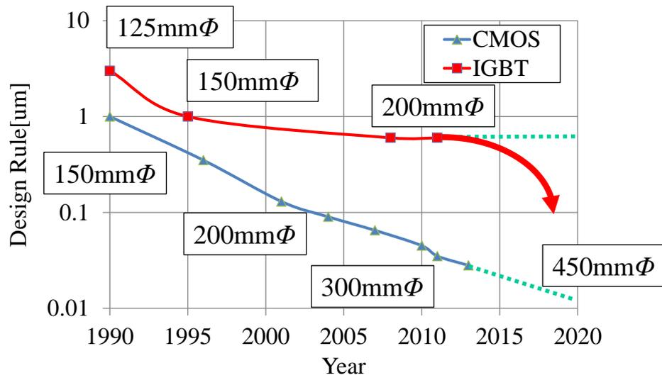
Figure 8. IGBT process direction. Keeping process compatibility with CMOS is needed.
